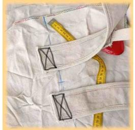
**3.5 Attach straps to backpack:** The roll-top of backpack is 20cm long so stitch shoulder straps onto back panel 20cm below top edge with a 'box x' stitch.
